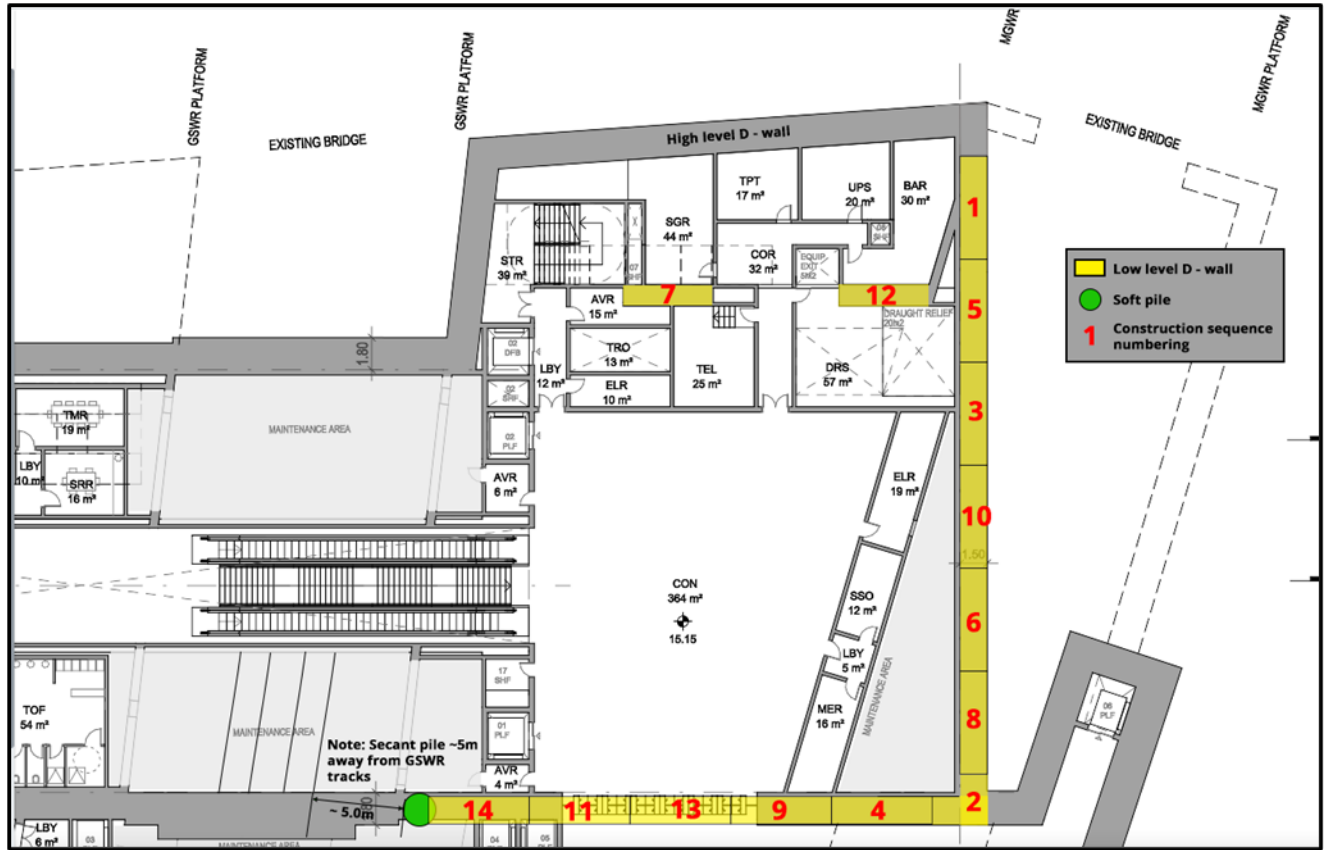
Figure 5.21: Diaphragm Wall Panel Arrangement and Sequence of Construction for the Low-Level South Side
