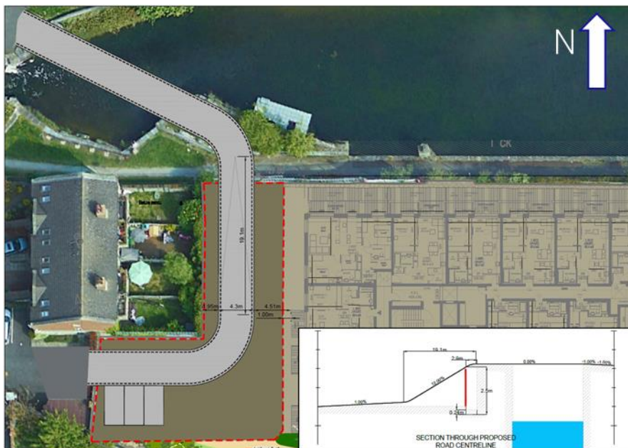
Figure 6.4 Proposed southern access to the temporary bridge
